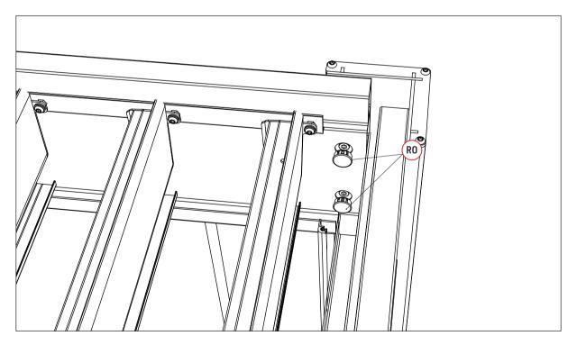
After confirming the dimensions, then fix the expansion bolts on the plate.
